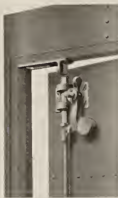
Showing Automatic Latch Engaging Bolt Head
