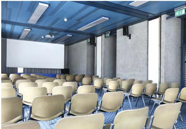
**Concentrated use in an Assembly occupancy may include chairs that are not fixed, and the occupant load factor is 7 net square feet per person.**
