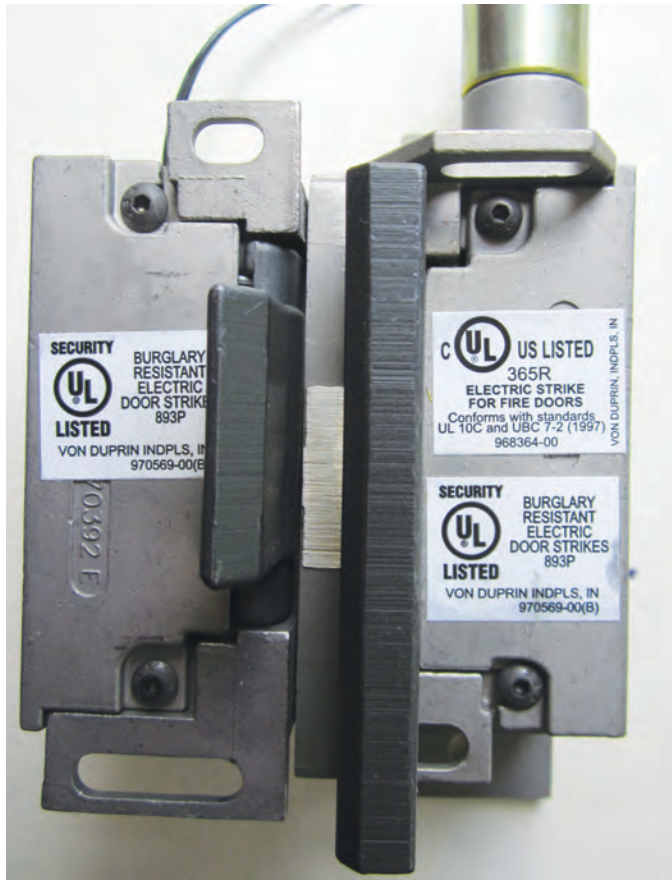
These fail-secure strikes have UL labels for fire and burglary, while the fail-safe strikes only have a UL label for burglary.
