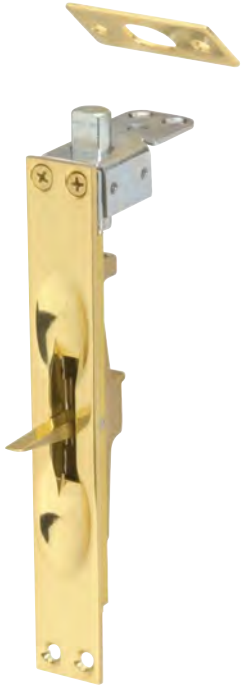
Manual flush bolts must be projected and retracted manually, so there are limitations regarding their use on fire doors and egress doors.
